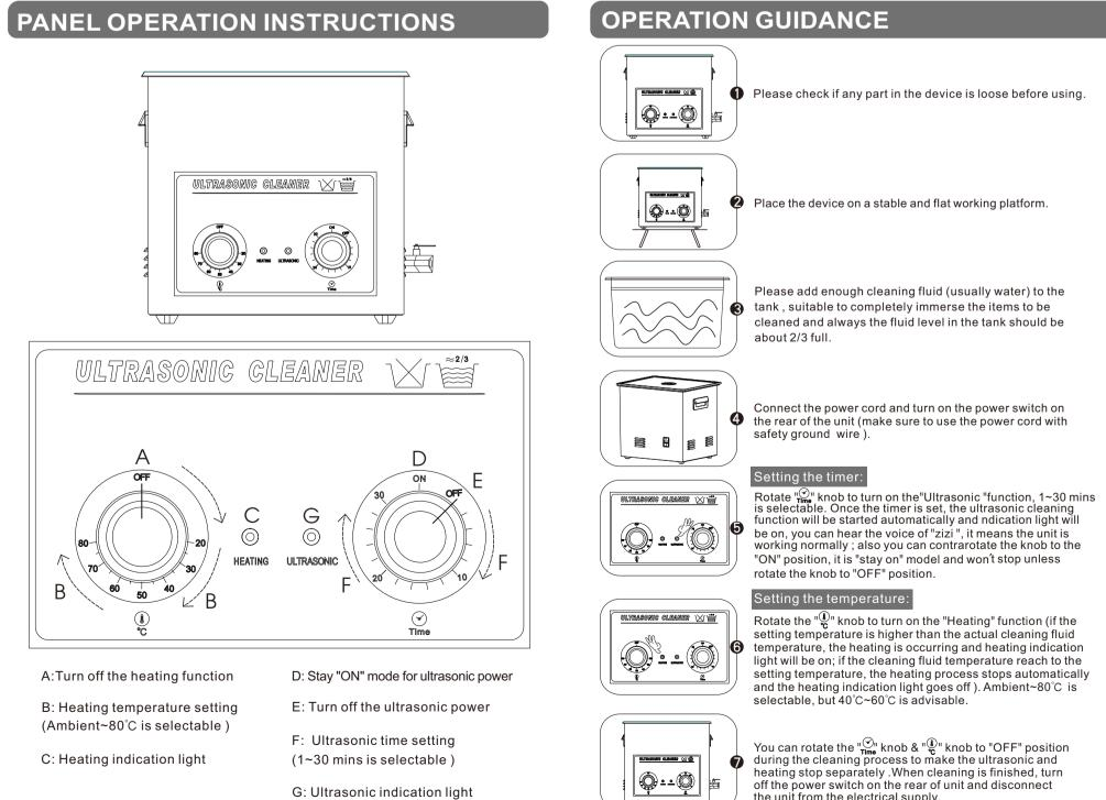
setting temperature, the heating process stops automatically and the heating indication light goes off ). Ambient~80°C is selectable, but 40°C~60°C is advisable. You can rotate the "Time knob & "C" knob to "OFF" position during the cleaning process to make the ultrasonic and heating stop separately .When cleaning is finished, turn off the power switch on the rear of unit and disconnect the unit from the electrical supply.
